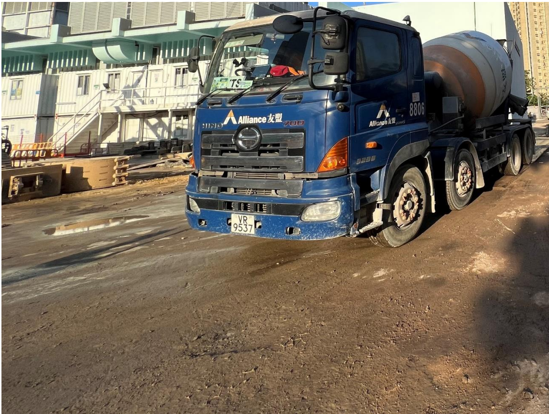
Figure 2.1: HINO EURO V Concrete Lorry Mixer (VR9537)
